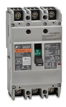
Fuji Electric molded case circuit breaker, 125A frame, 20A, 600 VAC / 250 VDC, 3-pole, characteristics, thermal magnetic, 30kA @ 480 VAC interrupting rating, panel mount. Line and load lug terminals and terminal covers included.
