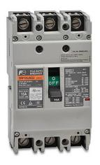
Fuji Electric molded case circuit breaker, 125A frame, 15A, 600 VAC / 250 VDC, 3-pole, characteristics, thermal magnetic, 30kA @ 480 VAC interrupting rating, panel mount. Line and load lug terminals and terminal covers included.
