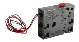
NITRA solenoid valve, 4-port (4-way), 2-position, single solenoid spring return, (1) 6mm PTC tubing inlet(s), (2) 6mm PTC tubing outlet(s), (1) 6mm PTC tubing exhaust(s), Cv=0.8, 120 VAC, 1.5VA, removable 18in pigtail.
