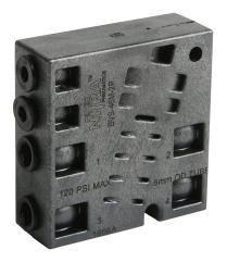
NITRA pilot valve, 4-port (4-way), 2-position, double air pilot, (1) 6mm push-to-connect inlet(s), (2) 6mm push-to-connect outlet(s), (1) 6mm PTC tubing exhaust(s), (2) 5/32in (4mm) push-to-connect tubing pilot(s), Cv=0.8.
