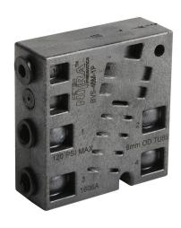
NITRA pilot valve, 4-port (4-way), 2-position, single air pilot spring return, (1) 6mm PTC tubing inlet(s), (2) 6mm PTC tubing outlet(s), (1) 6mm PTC tubing exhaust(s), (1) 5/32in (4mm) PTC tubing, Cv=0.8.
