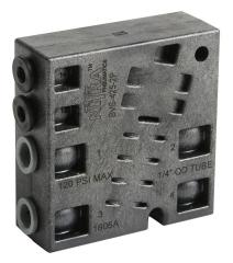
NITRA pilot valve, 4-port (4-way), 2-position, double air pilot, (1) 1/4in PTC tubing inlet(s), (2) 1/4in PTC tubing outlet(s), (1) 1/4in PTC tubing exhaust(s), (2) 5/32in (4mm) push-to-connect tubing pilot(s), Cv=0.8.
