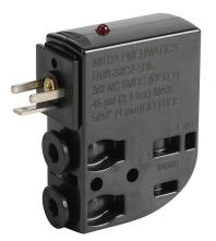
NITRA solenoid valve, 3-port (3-way), 2-position, N.C., single solenoid spring return, (1) 5/32in (4mm) PTC tubing inlet(s), (1) 5/32in (4mm) PTC tubing outlet(s), (1) vent hole exhaust(s), Cv=0.02, 5 VDC, 0.5W, 8mm DIN style wiring plug.
