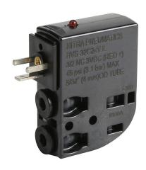
NITRA solenoid valve, 3-port (3-way), 2-position, N.C., single solenoid spring return, (1) 5/32in (4mm) PTC tubing inlet(s), (1) 5/32in (4mm) PTC tubing outlet(s), (1) vent hole exhaust(s), Cv=0.02, 3 VDC, 0.5W, 8mm DIN style wiring plug.
