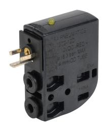
NITRA solenoid valve, 3-port (3-way), 2-position, N.C., single solenoid spring return, (1) 5/32in (4mm) PTC tubing inlet(s), (1) 5/32in (4mm) PTC tubing outlet(s), (1) vent hole exhaust(s), Cv=0.02, 12 VDC, 1.3W, 8mm DIN style wiring plug.
