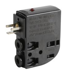
NITRA solenoid valve, 3-port (3-way), 2-position, N.C., single solenoid spring return, (1) 5/32in (4mm) PTC tubing inlet(s), (1) 5/32in (4mm) PTC tubing outlet(s), (1) vent hole exhaust(s), Cv=0.02, 12 VDC, 0.5W, 8mm DIN style wiring plug.
