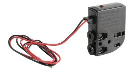
NITRA solenoid valve, 3-port (3-way), 2-position, N.C., single solenoid spring return, (1) 5/32in (4mm) push-to-connect inlet(s), (1) 5/32in (4mm) push-to-connect outlet(s), (1) vent hole exhaust(s), Cv=0.02, 3 VDC, 0.5W, removable 18in pigtail.
