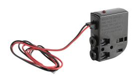
NITRA solenoid valve, 3-port (3-way), 2-position, N.C., single solenoid spring return, (1) 5/32in (4mm) PTC tubing inlet(s), (1) 5/32in (4mm) PTC tubing outlet(s), (1) vent hole exhaust(s), Cv=0.02, 3 VDC, 0.5W, removable 18in pigtail.
