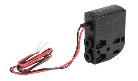
NITRA solenoid valve, 3-port (3-way), 2-position, N.C., single solenoid spring return, (1) 5/32in (4mm) PTC tubing inlet(s), (1) 5/32in (4mm) PTC tubing outlet(s), (1) vent hole exhaust(s), Cv=0.02, 120 VAC, 1.5VA, removable 18in pigtail.
