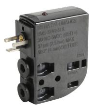
NITRA solenoid valve, 3-port (3-way), 2-position, N.O., single solenoid spring return, (1) 5/32in (4mm) PTC tubing inlet(s), (1) 5/32in (4mm) PTC tubing outlet(s), (1) vent hole exhaust(s), Cv=0.02, 5 VDC, 0.5W, 8mm DIN style wiring plug.
