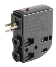
NITRA solenoid valve, 3-port (3-way), 2-position, N.O., single solenoid spring return, (1) 5/32in (4mm) PTC tubing inlet(s), (1) 5/32in (4mm) PTC tubing outlet(s), (1) vent hole exhaust(s), Cv=0.02, 3 VDC, 0.5W, 8mm DIN style wiring plug.
