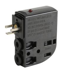
NITRA solenoid valve, 3-port (3-way), 2-position, N.O., single solenoid spring return, (1) 5/32in (4mm) PTC tubing inlet(s), (1) 5/32in (4mm) PTC tubing outlet(s), (1) vent hole exhaust(s), Cv=0.02, 24 VDC, 0.5W, 8mm DIN style wiring plug.
