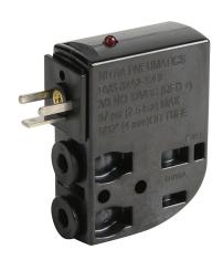
NITRA solenoid valve, 3-port (3-way), 2-position, N.O., single solenoid spring return, (1) 5/32in (4mm) PTC tubing inlet(s), (1) 5/32in (4mm) PTC tubing outlet(s), (1) vent hole exhaust(s), Cv=0.02, 12 VDC, 0.5W, 8mm DIN style wiring plug.
