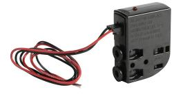
NITRA solenoid valve, 3-port (3-way), 2-position, N.O., single solenoid spring return, (1) 5/32in (4mm) PTC tubing inlet(s), (1) 5/32in (4mm) PTC tubing outlet(s), (1) vent hole exhaust(s), Cv=0.02, 5 VDC, 0.5W, removable 18in pigtail.
