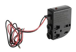
NITRA solenoid valve, 3-port (3-way), 2-position, N.O., single solenoid spring return, (1) 5/32in (4mm) PTC tubing inlet(s), (1) 5/32in (4mm) PTC tubing outlet(s), (1) vent hole exhaust(s), Cv=0.02, 3 VDC, 0.5W, removable 18in pigtail.
