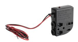
NITRA solenoid valve, 3-port (3-way), 2-position, N.O., single solenoid spring return, (1) 5/32in (4mm) PTC tubing inlet(s), (1) 5/32in (4mm) PTC tubing outlet(s), (1) vent hole exhaust(s), Cv=0.02, 12 VDC, 0.5W, removable 18in pigtail.
