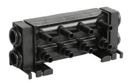
NITRA pneumatic modular valve manifold, fiberglass-reinforced thermoplastic, (4) stations, (2) 10mm push-to-connect tubing inlet(s), (2) 10mm push-to-connect tubing exhaust(s). For use with BVS-46M series valves.
