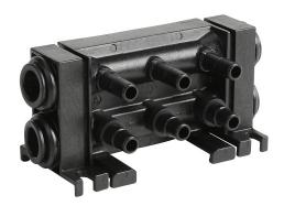
NITRA pneumatic modular valve manifold, fiberglass-reinforced thermoplastic, (3) stations, (2) 10mm push-to-connect tubing inlet(s), (2) 10mm push-to-connect tubing exhaust(s). For use with BVS-46M series valves.
