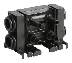
NITRA pneumatic modular valve manifold, fiberglass-reinforced thermoplastic, (2) stations, (2) 10mm push-to-connect tubing inlet(s), (2) 10mm push-to-connect tubing exhaust(s). For use with BVS-46M series valves.
