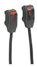
Autonics photoelectric sensor, rectangular, polybutylene terephthalate housing, through-beam pair, visible red, 0-1m sensing distance, 10.8-26.4 VDC operating voltage, light-on, NPN, 3-wire, pigtail.
