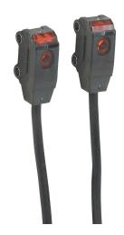
Autonics photoelectric sensor, rectangular, polybutylene terephthalate housing, through-beam pair, visible red, 0-1m sensing distance, 10.8-26.4 VDC operating voltage, light-on, PNP, 3-wire, pigtail.
