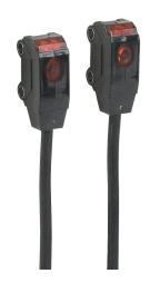
Autonics photoelectric sensor, rectangular, polybutylene terephthalate housing, through-beam pair, visible red, 0-1m sensing distance, 10.8-26.4 VDC operating voltage, dark-on, NPN, 3-wire, pigtail.
