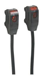
Autonics photoelectric sensor, rectangular, polybutylene terephthalate housing, through-beam pair, visible red, 0-1m sensing distance, 10.8-26.4 VDC operating voltage, dark-on, PNP, 3-wire, pigtail.
