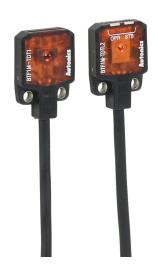
Autonics photoelectric sensor, rectangular, polybutylene terephthalate housing, through-beam pair, visible red, 0-1m sensing distance, 10.8-26.4 VDC operating voltage, light-on, NPN, 3-wire, pigtail.
