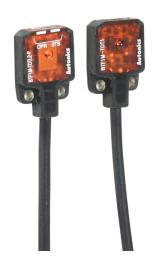
Autonics photoelectric sensor, rectangular, polybutylene terephthalate housing, through-beam pair, visible red, 0-1m sensing distance, 10.8-26.4 VDC operating voltage, light-on, PNP, 3-wire, pigtail.
