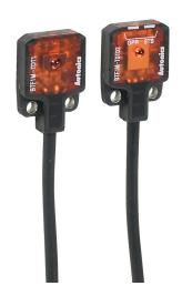
Autonics photoelectric sensor, rectangular, polybutylene terephthalate housing, through-beam pair, visible red, 0-1m sensing distance, 10.8-26.4 VDC operating voltage, dark-on, NPN, 3-wire, pigtail.
