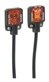
Autonics photoelectric sensor, rectangular, polybutylene terephthalate housing, through-beam pair, visible red, 0-1m sensing distance, 10.8-26.4 VDC operating voltage, dark-on, PNP, 3-wire, pigtail.
