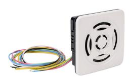
Patlite audible alarm, 85 dB at 1m, 246 Hz to 2.9 kHz tone frequency, (15) selectable tone(s), 12-24 VDC, panel or surface mount, polycarbonate housing, off-white, IP54.
