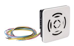
Patlite audible alarm, 85 dB at 1m, 246 Hz to 2.9 kHz tone frequency, (15) selectable tone(s), 12-24 VDC, panel or surface mount, polycarbonate housing, off-white, IP54.
