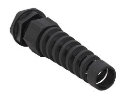
Bimed cable gland, PG16 thread type, polyamide, black, accepts 10 to 14mm diameter cable, IP68, with strain relief. Package of 5. Mounting hardware included.
