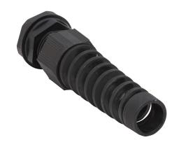
Bimed cable gland, PG13.5 thread type, polyamide, black, accepts 6 to 12mm diameter cable, IP68, with strain relief. Package of 5. Mounting hardware included.
