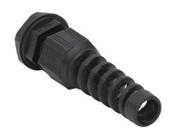
Bimed cable gland, PG9 thread type, polyamide, black, accepts 4 to 8mm diameter cable, IP68, with strain relief. Package of 5. Mounting hardware included.
