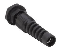
Bimed cable gland, PG7 thread type, polyamide, black, accepts 3 to 6.5mm diameter cable, IP68, with strain relief. Package of 5. Mounting hardware included.
