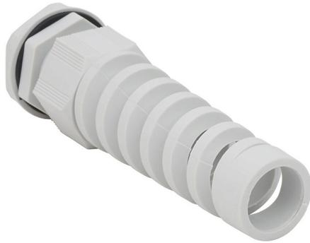
Bimed cable gland, PG21 thread type, polyamide, light gray, accepts 13 to 18mm diameter cable, IP68, with strain relief. Package of 5. Mounting hardware included.
