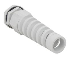
Bimed cable gland, PG21 thread type, polyamide, light gray, accepts 13 to 18mm diameter cable, IP68, with strain relief. Package of 5. Mounting hardware included.
