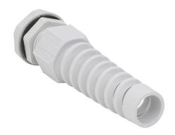
Bimed cable gland, PG13.5 thread type, polyamide, light gray, accepts 6 to 12mm diameter cable, IP68, with strain relief. Package of 5. Mounting hardware included.
