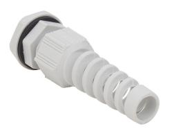
Bimed cable gland, PG9 thread type, polyamide, light gray, accepts 4 to 8mm diameter cable, IP68, with strain relief. Package of 5. Mounting hardware included.
