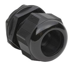
Bimed cable gland, 1in NPT thread type, polyamide, black, accepts 18 to 25mm diameter cable, IP68. Package of 5. Mounting hardware included.
