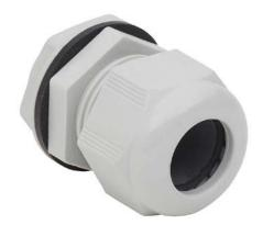
Bimed cable gland, 3/4in NPT thread type, polyamide, light gray, accepts 13 to 18mm diameter cable, IP68. Package of 5. Mounting hardware included.
