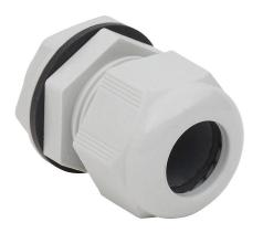
Bimed cable gland, 3/4in NPT thread type, polyamide, light gray, accepts 13 to 18mm diameter cable, IP68. Package of 5. Mounting hardware included.
