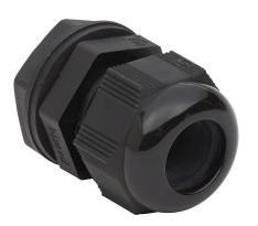
Bimed cable gland, 1/2in NPT thread type, polyamide, black, accepts 10 to 14mm diameter cable, IP68. Package of 5. Mounting hardware included.
