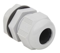
Bimed cable gland, 1/2in NPT thread type, polyamide, light gray, accepts 10 to 14mm diameter cable, IP68. Package of 5. Mounting hardware included.
