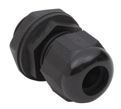
Bimed cable gland, 1/2in NPT thread type, polyamide, black, accepts 6 to 12mm diameter cable, IP68. Package of 5. Mounting hardware included.
