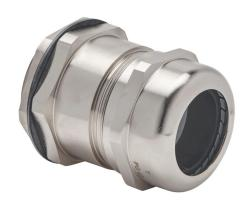
Bimed EMC cable gland, PG42 thread type, nickel-plated brass, accepts 30 to 38mm diameter cable, IP68. Mounting hardware included.
