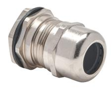
Bimed EMC cable gland, PG21 thread type, nickel-plated brass, accepts 10 to 18mm diameter cable, IP68. Package of 5. Mounting hardware included.
