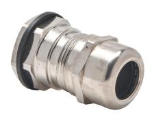
Bimed EMC cable gland, PG16 thread type, nickel-plated brass, accepts 7.5 to 14mm diameter cable, IP68. Package of 5. Mounting hardware included.
