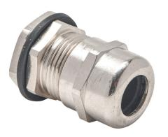
Bimed EMC cable gland, PG13.5 thread type, nickel-plated brass, accepts 6 to 12mm diameter cable, IP68. Package of 5. Mounting hardware included.
