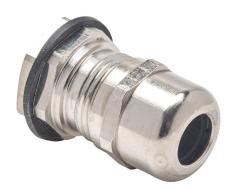
Bimed EMC cable gland, PG11 thread type, nickel-plated brass, accepts 5 to 10mm diameter cable, IP68. Package of 5. Mounting hardware included.
