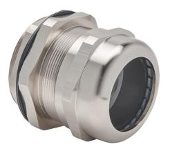
Bimed EMC cable gland, PG48 thread type, nickel-plated brass, accepts 34 to 44mm diameter cable, IP68. Mounting hardware included.
