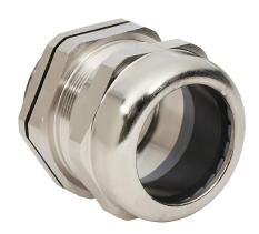
Bimed cable gland, PG48 thread type, nickel-plated brass, accepts 34 to 44mm diameter cable, IP68. Mounting hardware included.
